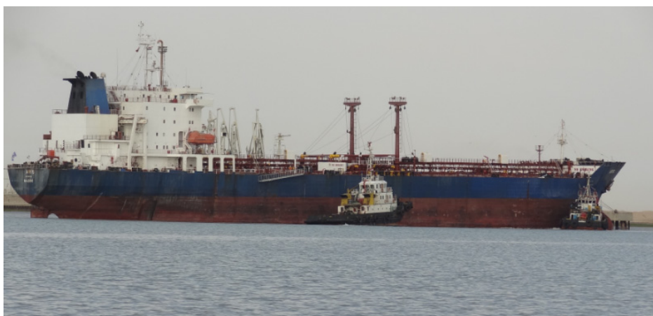
Photograph 9.5: Tugs manoeuvring a tanker into a berth
