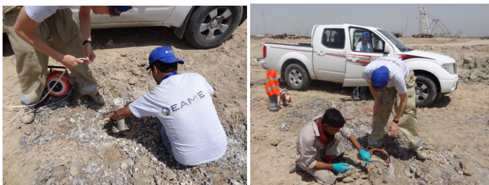
Photograph 7.2: BH03 being dipped using a groundwater interface probe and training Iraqi personnel to purge the monitoring wells
