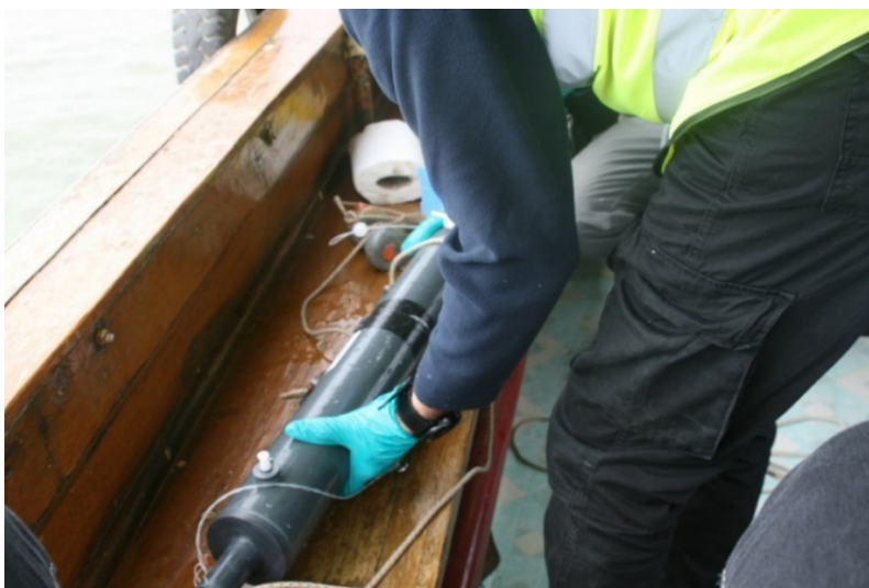
Photograph 7.3: Niskin Water Sampler
