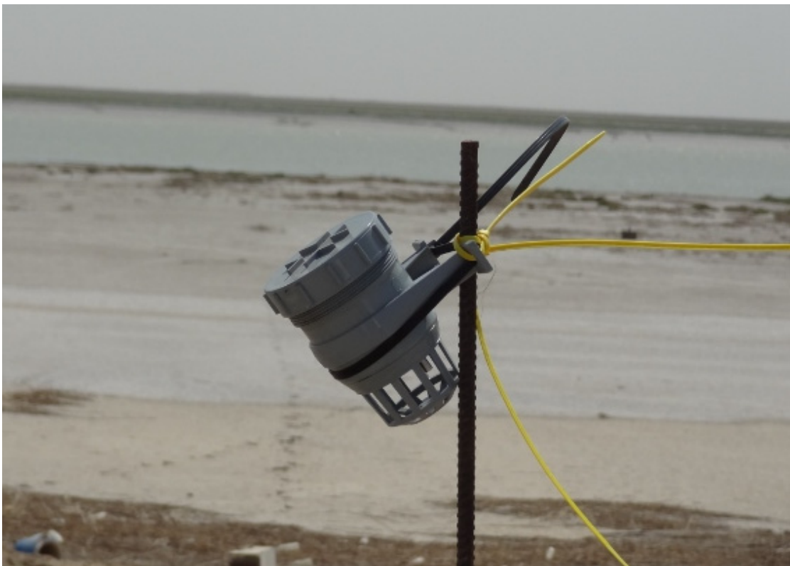
Photograph 5.2: Passive Tube Monitoring Shelter
